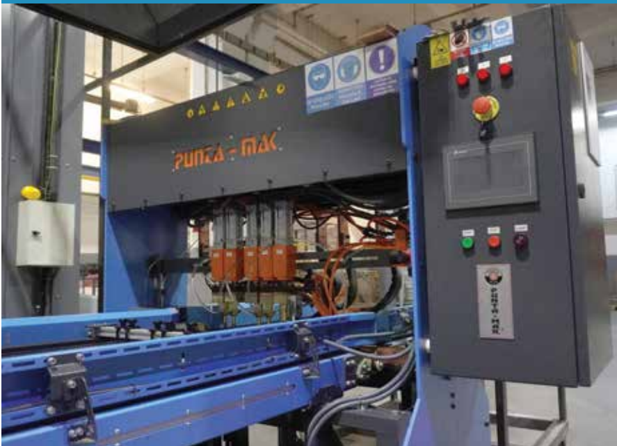
Automatic Spot Welding Machine
