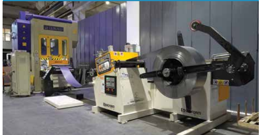
Sheet Metal Roll Opener and Straightener
